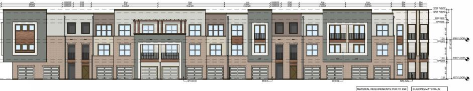
BRICK: 2,040 S.F.- 18% STUCCO: 3,260 S.F.- 59% SIDING: 170 S.F.- 3% TOTAL: 5,470 S.F.-100% 80% MIN. OTHER MATERIALS: PER UDC APPENDIX F STUCCO: (EXCLUSIVE OF MASONRY) 60% MAX GLAZING: 1,060 S.F.- 16%
